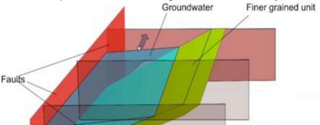
In the above illustration, provided by DTSC, we can see how faults can act as a contamination pathway. In addition the groundwater flow of the San Fernando Valley is from the Simi Hills to the east, fed by contaminated runoff and groundwater seeps.
