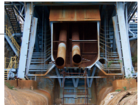
This Bravo test stand was used for test-firing engines with liquid fuel (kerosene). TCE was used to flush the engines before and after each test. This photo shows the bottom of the test stand.
